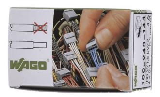
Junction box terminal 4-wire terminal 243-144 Number of clamping points 4, cable diameter 0.4 ... 0.5mm, color transparent, rated voltage 100V, nominal current 6A, suitable for solid conductors, AWG range 26 ... 24, MICRO junction box terminal for solid Conductor Ø 0.8 mm 4 conductors Housing color transparent Lid color light gray Ambient temperature max. 60°C
