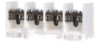
Power distribution block 4-p screw clamp Number of poles 4, Nominal current 80A, Connection type Screwing, Mounting method DIN rail, Number of connections total 20, Number of connections < 6 mm² 0, Number of connections 10 mm² 0, Number of connections 16 mm² 16, Number of connections 25 mm² 4, Number of connections > 25 mm² 0, Height 62mm, Width 119mm, Depth 49mm
